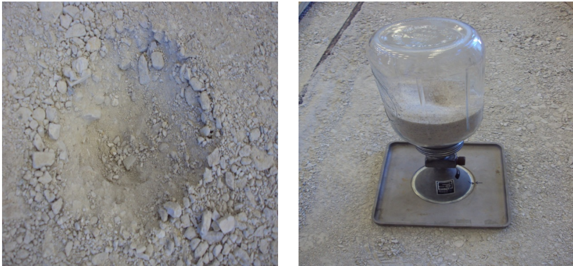
Figure 7-12 In Place Density Testing Using the Sand Cone Method
