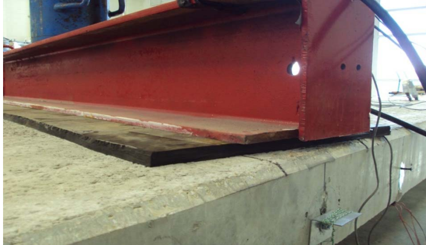
Figure 7-25 Spreader Beam with Neoprene Pad
