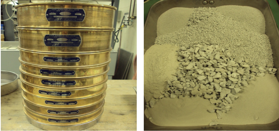
Figure 7-9 Sieves and Graded Material
