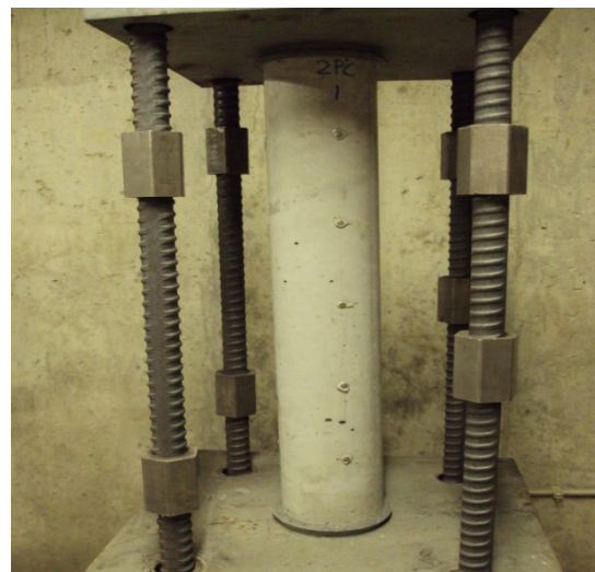
Figure 7-2 DEMEC Point Locations and Cylinder Loaded in Creep Frame [21]
