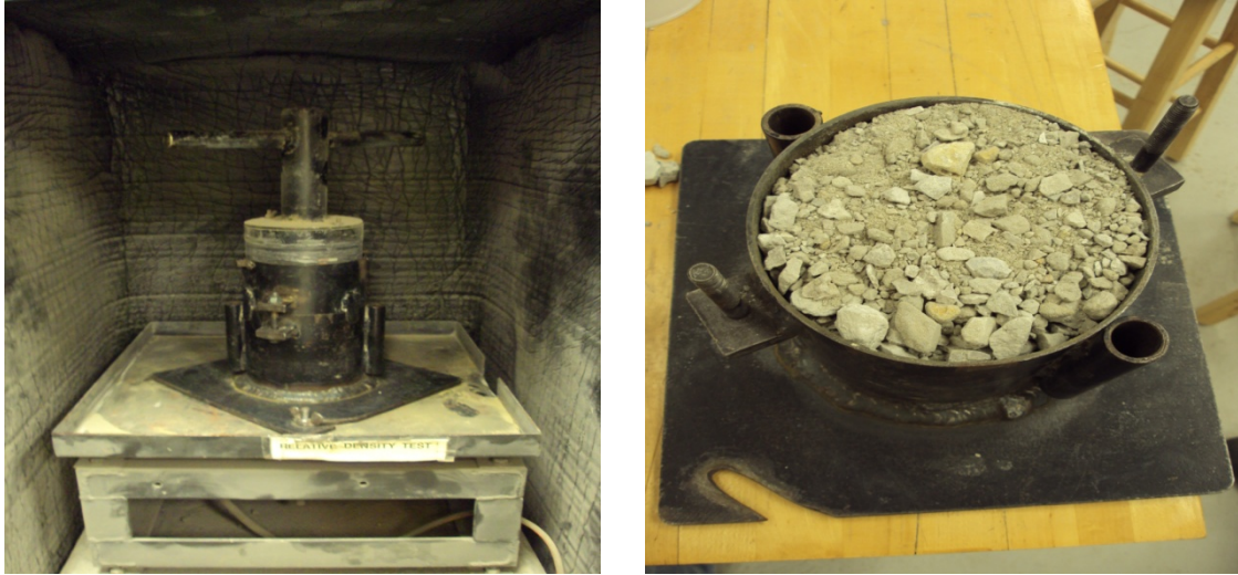
Figure 7-11 Vibratory Table and Compaction Mold
