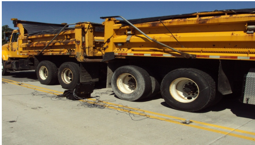
Figure 6-2 Overloading left lane for the BAS on Bridge A7890
