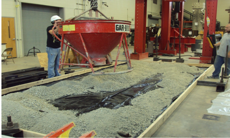
Figure 7-7 Placement of the aggregate base
