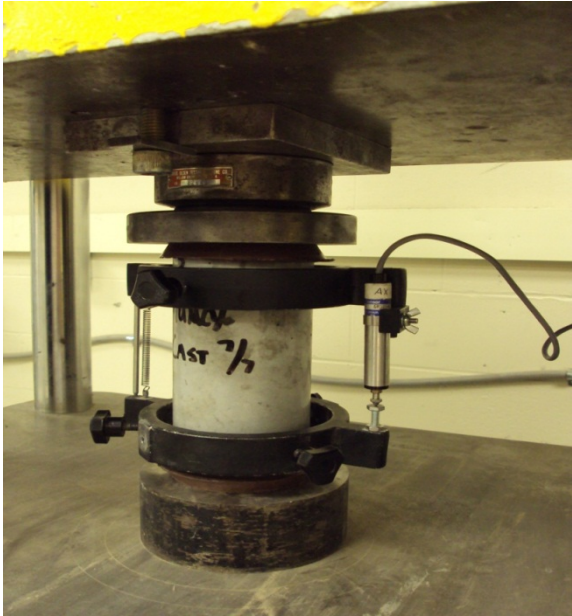
Figure 7-1 Test setup for compressive strength in the Tinius-Olsen
