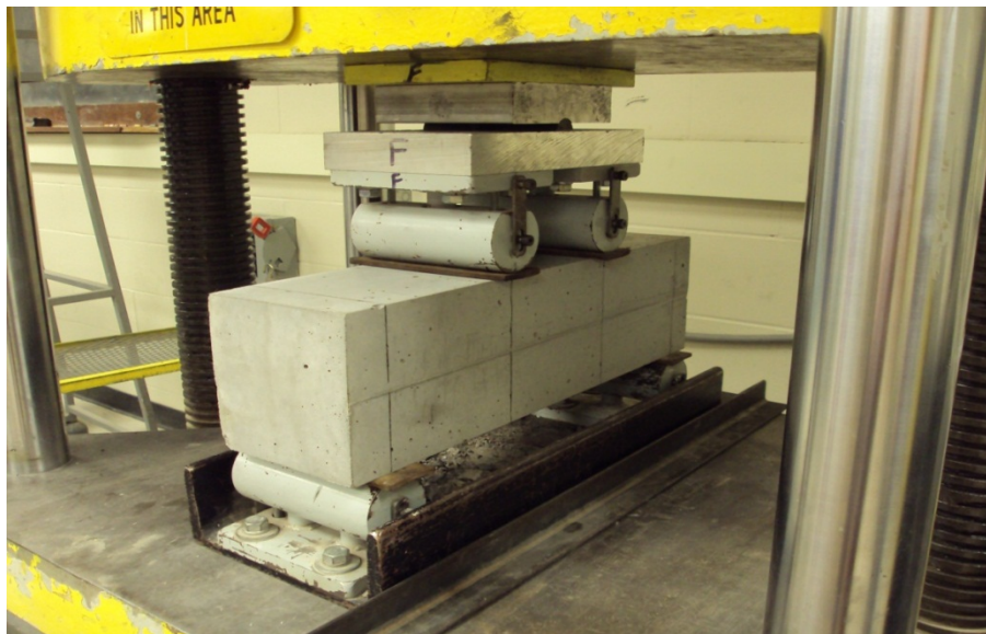
Figure 7-4 MOR Test Setup
