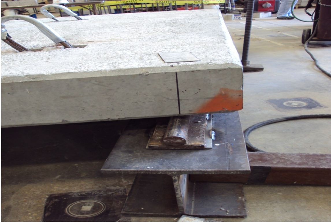
Figure 7-21 Panel End Support When Testing to Failure
