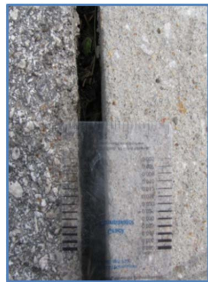
Figure 6-44 Gap between the approach pavement and approach slab at north shoulder, center & south shoulder respectively on Bridge A7890 at Final Site Inspection
