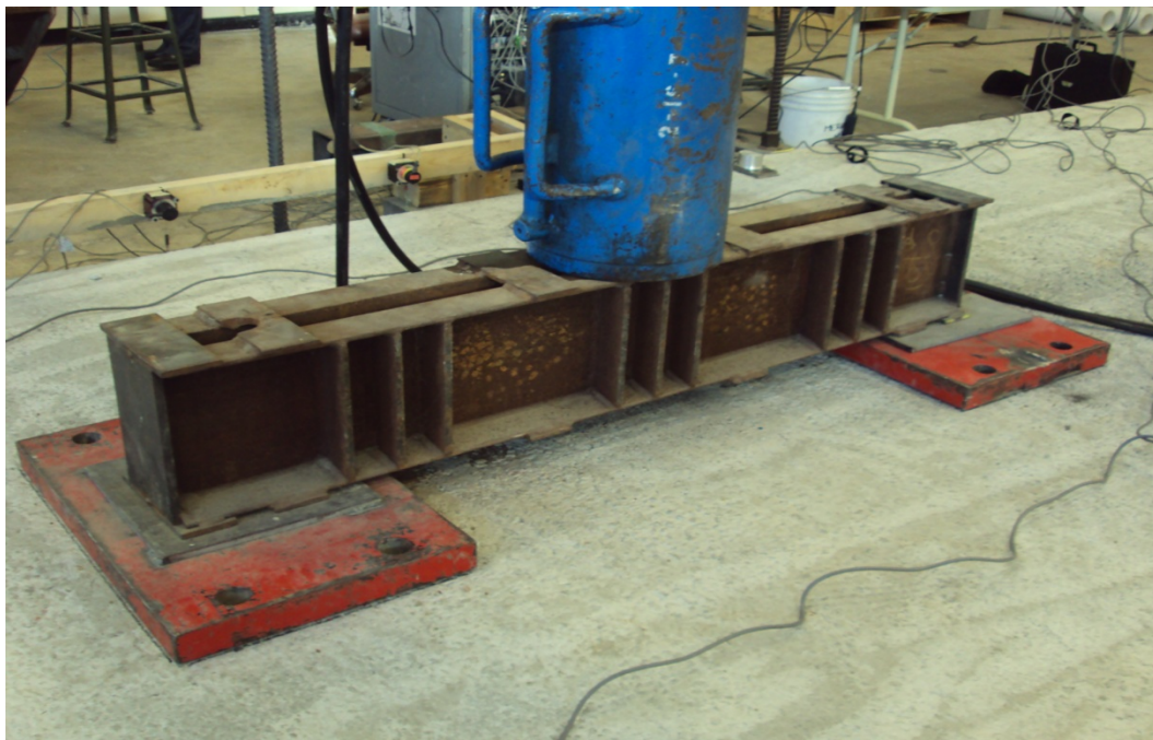
Figure 7-19 Spreader Beam and Bearing Plates
