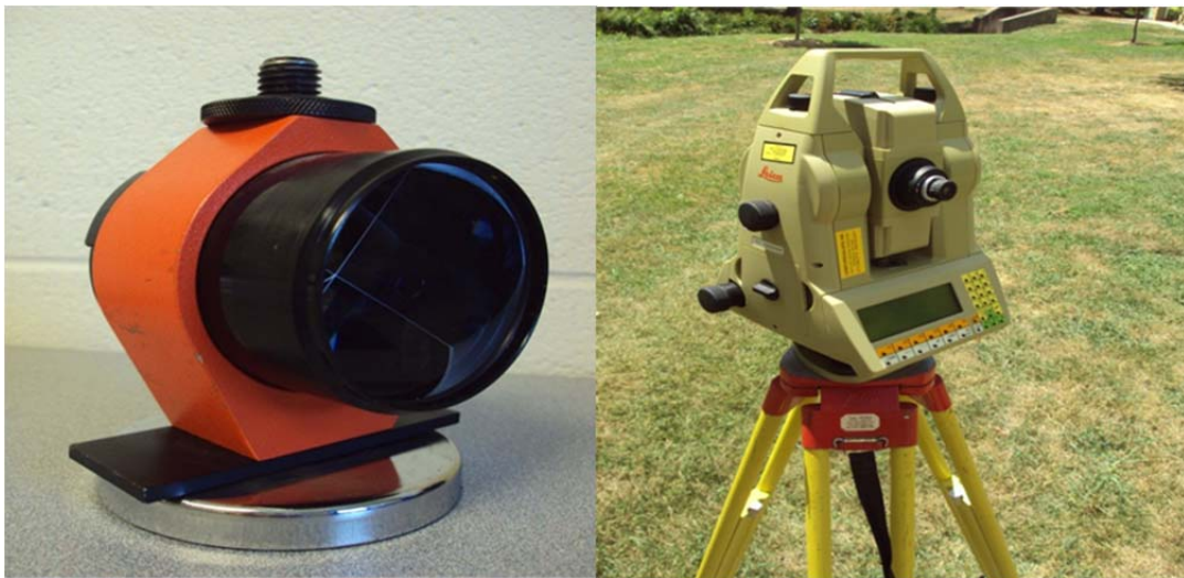
Figure 3-1 Surveying prism (left) and the Total Station (right)
