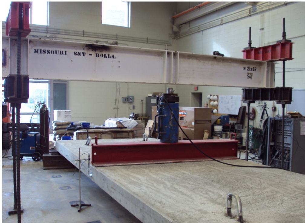
Figure 7-22 Testing Apparatus for Testing Panel to Failure
